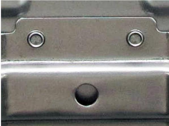
Figure 2 shows the micrograph of a ClinchRivet<sup>®</sup>-Joint
